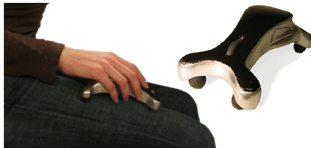
Figure 3: Users can operate thigh mouse without a desk. Retractable rubber feet prevent it from slipping.
