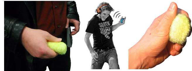
Figure 4: Soap is a combination of mouse and mouse pad in a single device [1]. An optical sensor inside the device is looking outwards. As the user drags the hull across the core, the optical sensor perceives the motion. Unlike accelerometer-based solutions, shaking the device does not affect input, allowing users to use soap while running or exercising.
