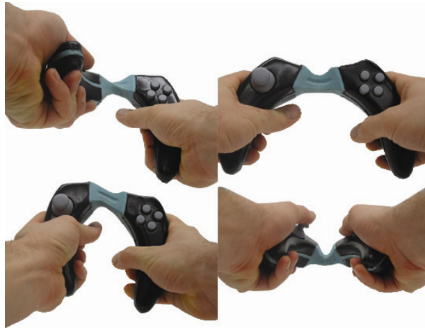
Figure 6: The D7 game controller's center joint offers more degrees of freedom than MS Side Winder Dual Strike [4]. Operating the joint is designed to require physical effort. The actions shown are left/right, forward/back, shear, & up/down.
