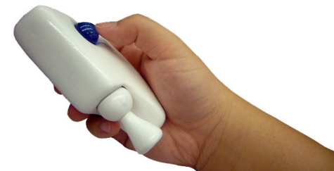
Figure 5: Users click the mobile trackball guppy navigator by tapping its white sensor stick against the user’s arm, a table, or a wall.
