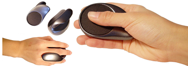
Figure 2: The brush is a one-handed touchpad designed for mobile use. The handle in the back of the device makes sure it stays put during physical activity.
